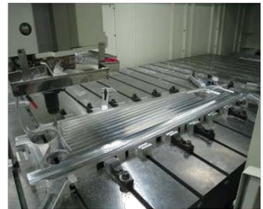
**CNC Machining Processes (with 99.5% Ethanol as lubricant)**
