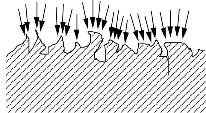
Resulting surface has reduced peaks, reduced surface area, and reduced outgassing
