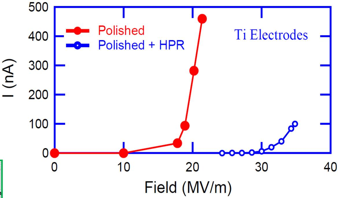
*HPR approved to be very effective to remove field emitters for Cornell ERL DC gun structure*
